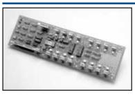
The MAI-16 uses 4 consecutive METRABUS addresses within the METRABUS 64-bit address space. This allows up to 16 MAI-16 boards (256 analog input points) to be controlled by a single METRABUS driver board. Writing to the MAI-16 addresses initiates conversions, controls input ranges and selects the channel to sample. Reading from the MAI-16 board address +0 will return the MSBs of the conversion while reading the board address +1 will return the LSBs.
